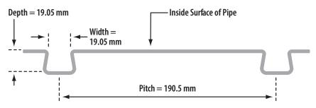
Tolerances shall be as noted in CSA G401 and/or ASTM A760
